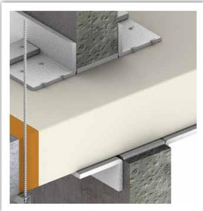
Wall penetration of the PROMAPAIN ® FD fire resisting duct system
